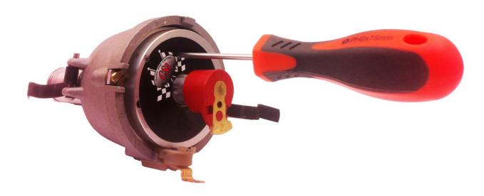
Changes the curves with a small philips screw driver.
