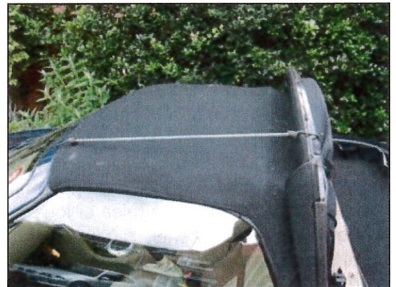
Figure 24, Hold spar in position.
