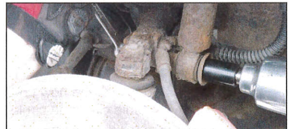
Figure 3, Note the correct positions of the brake hose clamp, spacer and two washers.
